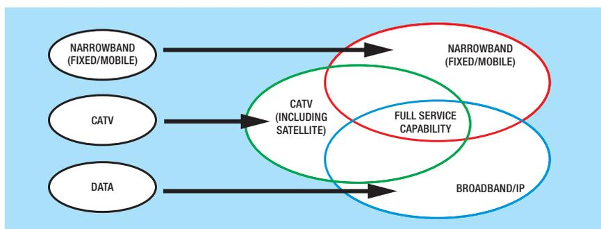
Figure 2—Network evolution. Besides the narrowband and TV broadcast networks a broadband/IP network is being established. The different networks are becoming interlinked and will have 'full service' capabilities
