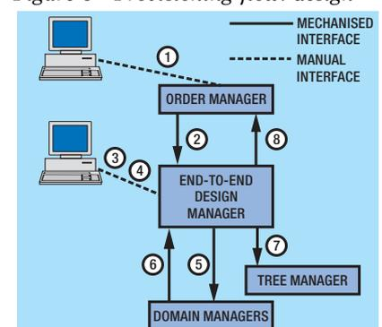
order manager captures the request in the form of a service order and initiates the appropriate provisioning task model.
