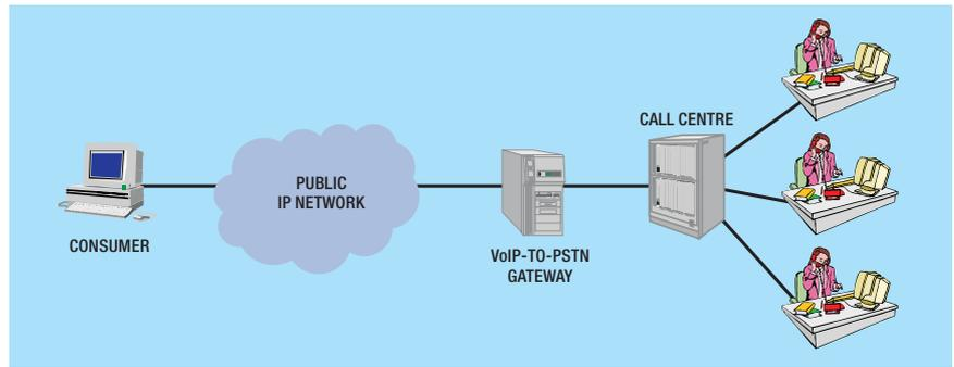
Figure 5—VoIP architecture for customer contact
