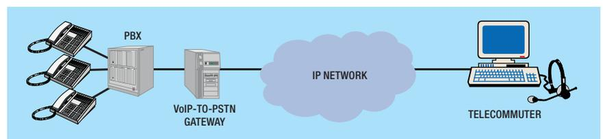
The architecture is very similar to the VoIP architecture used for customer contact. The only difference is that telecommuters have to log on to the gateway before they can use their PCs as telephones.
