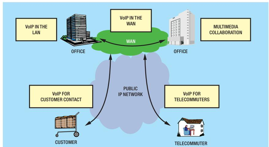
Figure 3—Architecture of a company network using VoIP over the LAN
