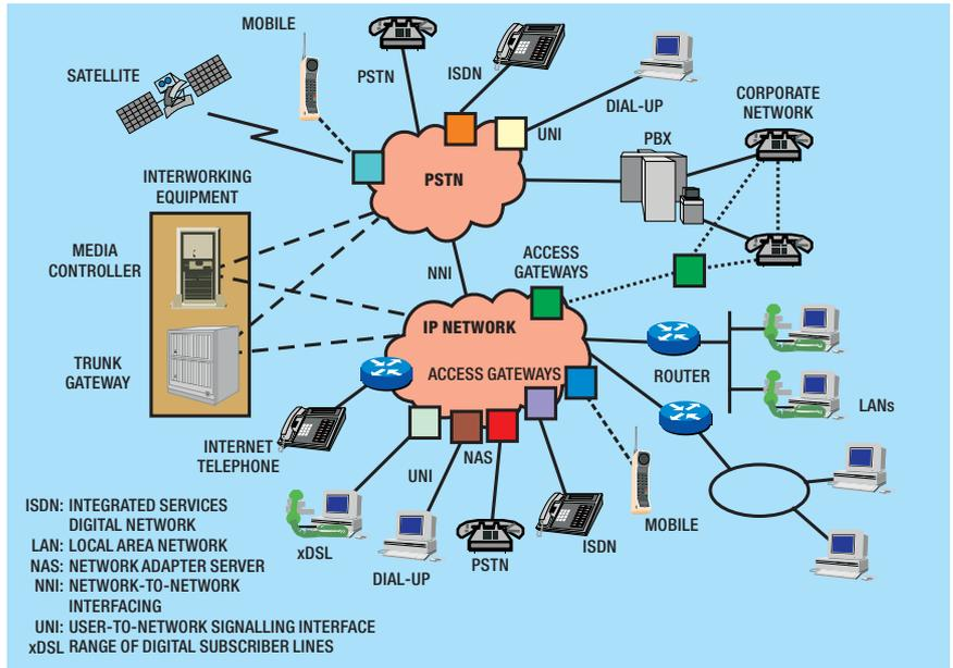
Figure 3—Signalling and control architecture for current VoIP
