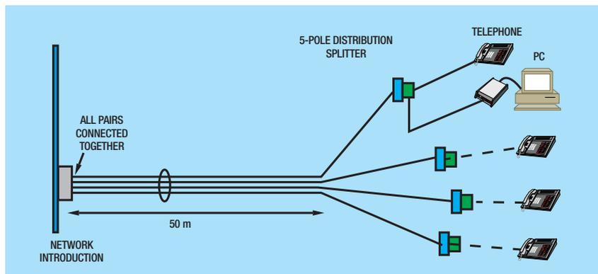
Then one items of POTS equipment was consecutively installed on each of the remaining wall sockets.
