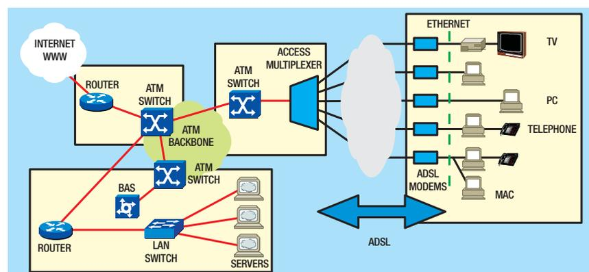
from different clients and to map them on to a dedicated interface to the ATM backbone. This can be an STM-1 interface, an E3 interface or multiple E1 interfaces, depending on the expected load on the specific DSLAM.
