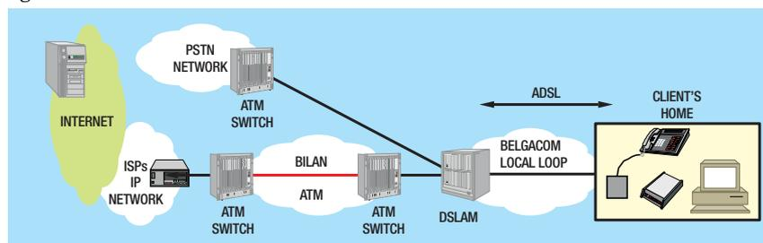
Figure 3—Connecting a DSLAM to the network by 'subtending'
