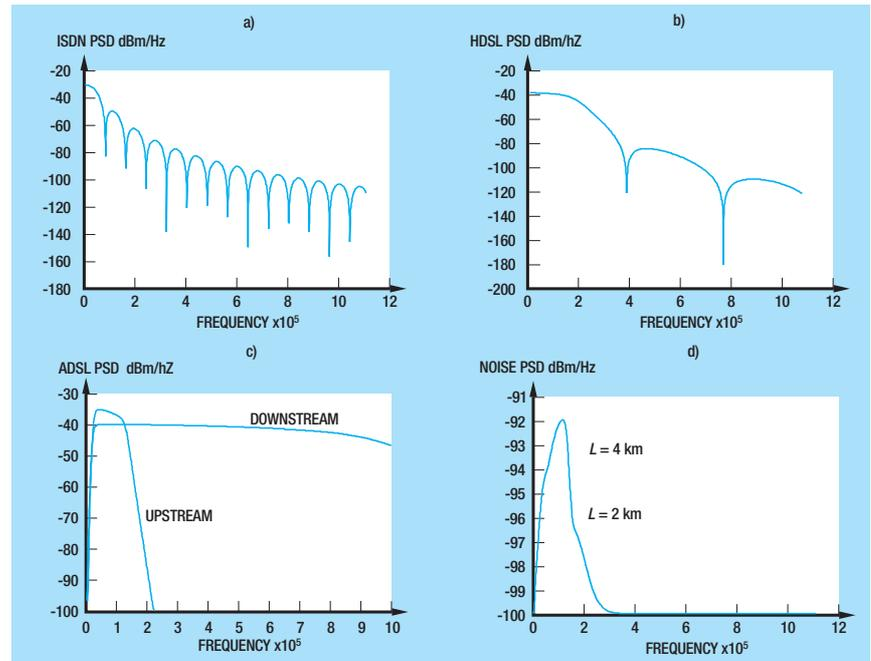
Figure 4—Power spectral densities of: (a) ISDN BRA; (b) HDSL; (c) ADSL up-stream and downstream; (d) NEXT+FEXT+ additive white Gaussian noise (AWGN)
